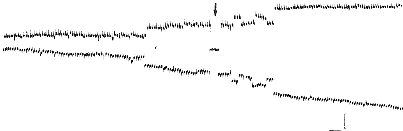
Fig. 6. Temporal increase of the macroscopic conductance G_0 after addition of surfactin ( 1.0 \mu\text{M} ) to the aqueous phase. The trace represents the voltage recorded by the Keithley electrometer (across a 10^8 \Omega resistor) following application of a 10 mV peak to peak alternating voltage across the membrane in series with the Keithley resistor. The salt was NaCl at 0.5 M. At the arrow, the surfactin was increased to 2.6 \mu\text{M} . The vertical bar represents 0.6 mV and the horizontal bar, 1 min.
